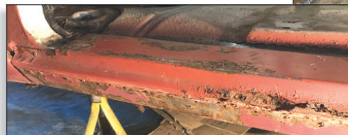
Above, just a small portion of the rust that Brad found awaiting him. Below, the rusted front rocker, and right, Brad's driver rocker mock-up
