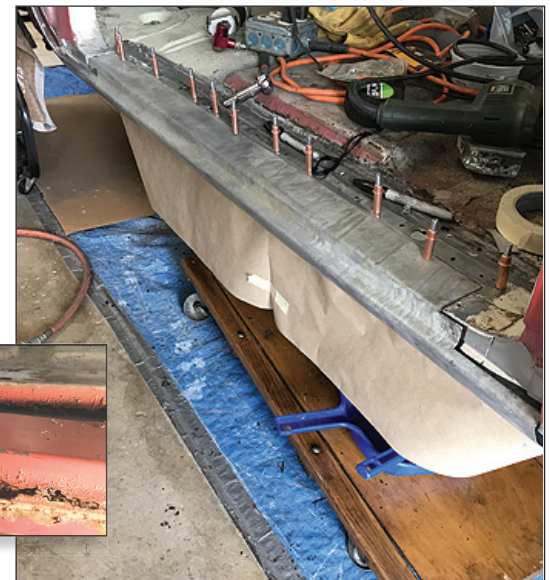
Above, just a small portion of the rust that Brad found awaiting him. Below, the rusted front rocker, and right, Brad's driver rocker mock-up
