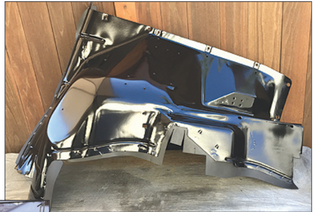
Above left: finished front electric; above right, restored inner fender; left, back from paint and ready to finish
