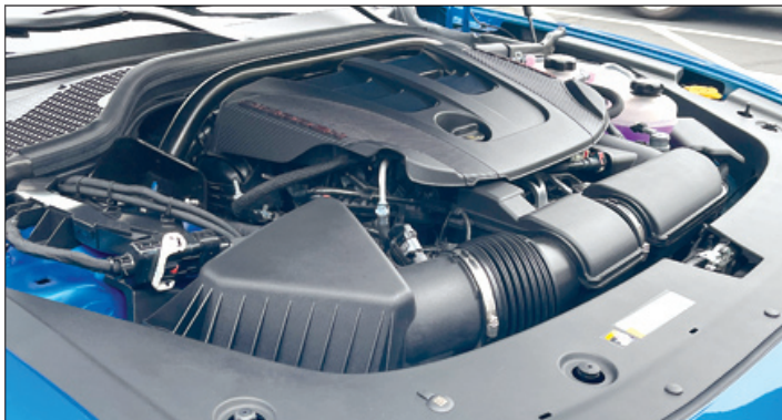
Modern vs Classic: Above, the new 550HP Hurricane engine in the 2026 3.0L Twin Turbo SixPack (and all-gas) Charger R/T, and below, Bill Baugh's 1966 Satellite Hemi. Asked by Dave Stall if he would ever want to work on the Hurricane? "Hell, no!"
