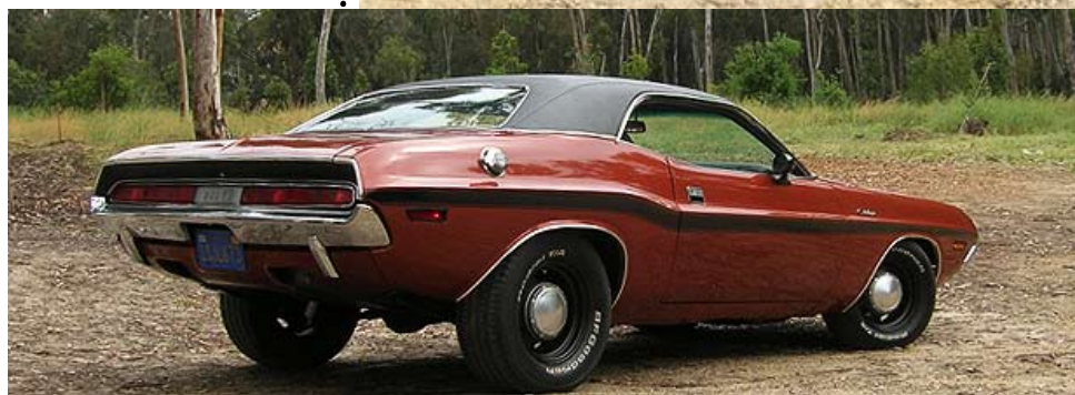
Steve removed the S/E rear window plug in favor of the larger standard rear window and rebuilt the front end. He and Dalis applied the black vinyl roof and decals. Steve also added "new bumpers, Cop Car wheels and dog dishes with 275/60x15's out back and 235/60x15's up front. The original disk brakes stop the car real well.
