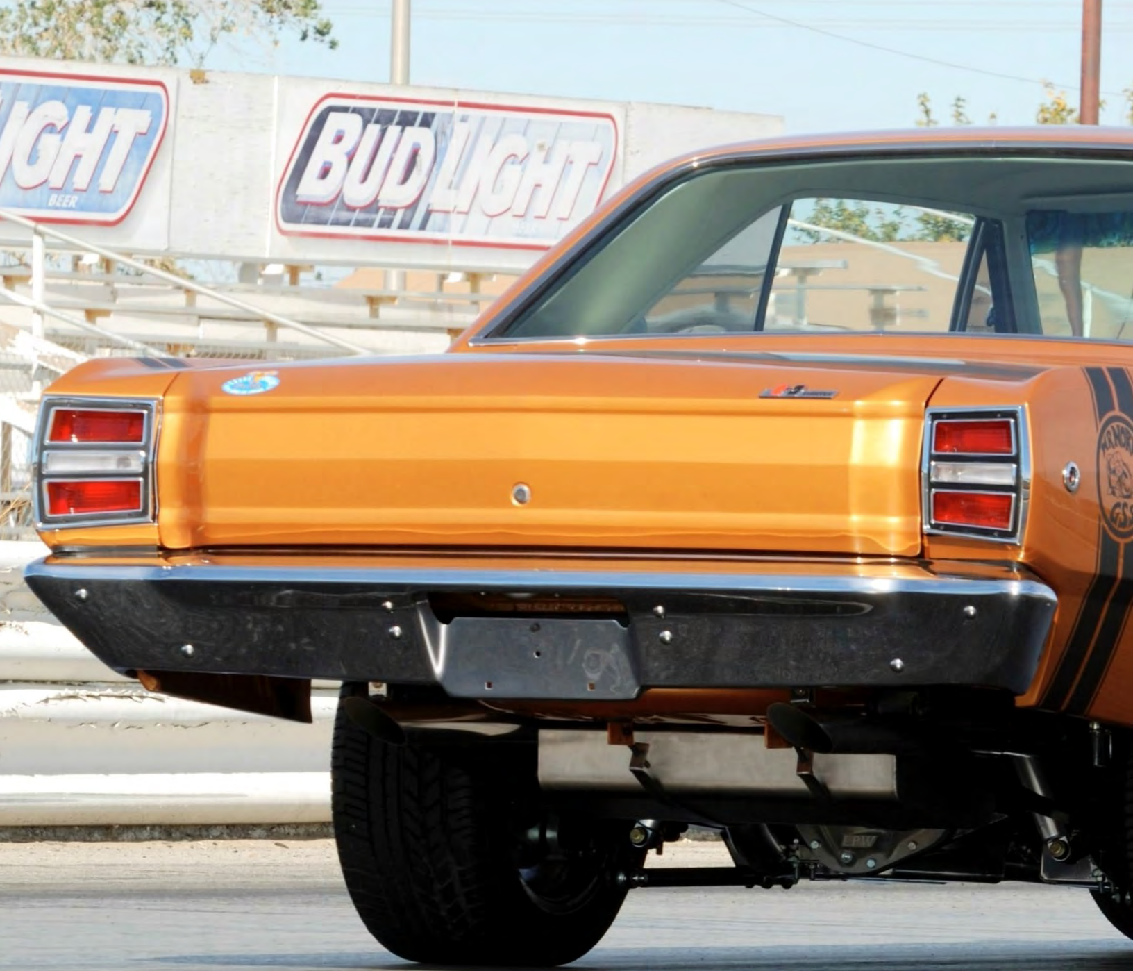
The GSS Hemi Dart shows off its “Run with the Scat Pack” ‘68 style split stripe. Look closely and you can see the stainless steel fuel tank, the LPW stud girdle on the Strange 60 rear end and the electric dumps.
