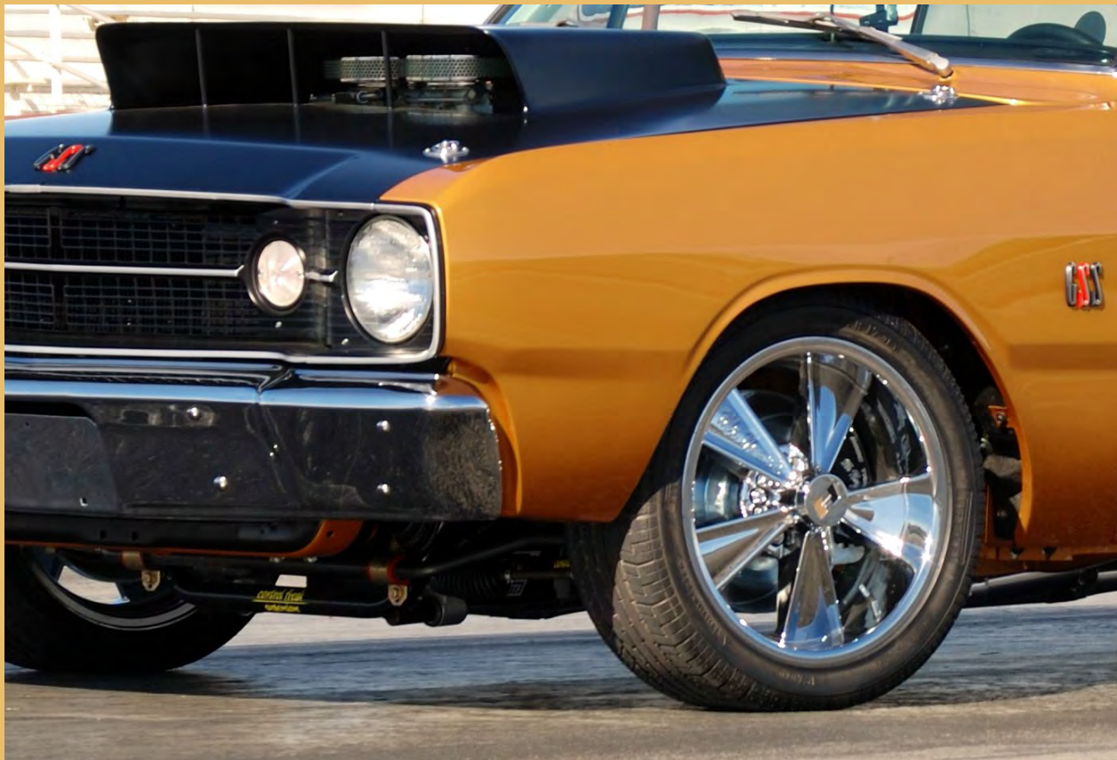
Mr. Norm's original GSS lettering in black, red, black combination adorn the front fenders and hood, just as they did back in 1968. Rolling stock consists of 17-inch Hurst style wheels by Oasis and Pirelli P-Zero Assimetrico tires. Right behind the wheels are SSBC Tri Power calipers and 13-inch Big Bite slotted rotors. Peeking through the black Super Stock lift off hood are a pair of Holley Hemi four barrel carbs.
