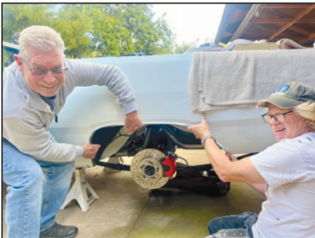
Brad and Shawn shaping, test fitting and marking drill points for mounting fender trim
