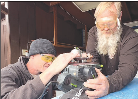
3. Cory and Tim grinding down center cap studs. After they drilled out all four wheels (5 studs/cap), the assembly line ramped up production
