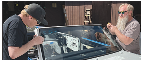
Cameron and Tim install the DePauw Dart's windshield
