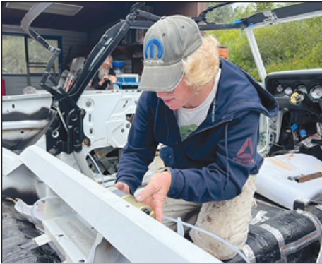
1. Shawn installing hydraulic motor and plumbing for the convertible top, before joining the wheels project
