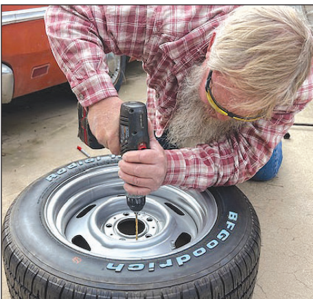
4. Tim had to drill out three additional holes per wheel
