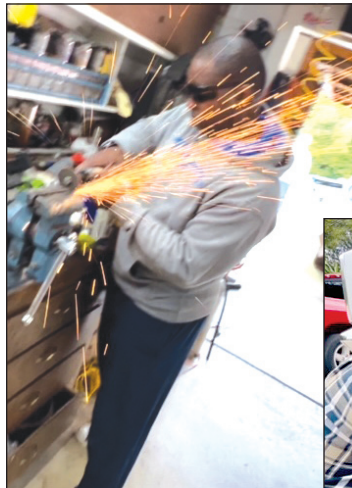
5. Since the center caps were reduced in length, 13 more bolts needed to be shortened and tapered. Jonathan doing the honors, above
